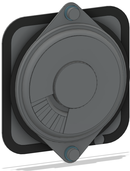
Fig. 20. Speaker and grille module viewed from inside. The mounting stack is retained.
