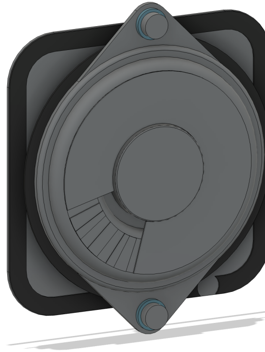
Fig. 27. Speaker, gasket, grille blank and hardware preserve the existing stack.
